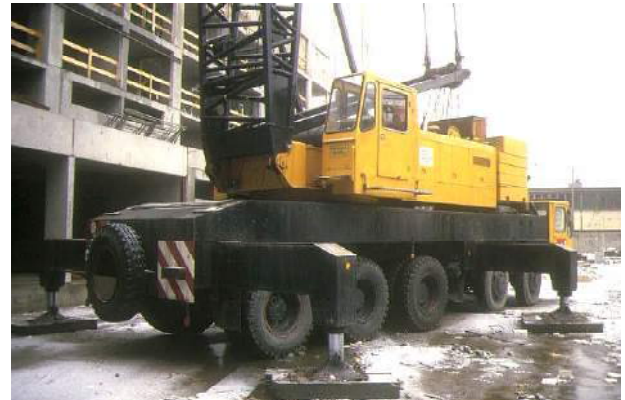
Below - LT3000 98 ton of 1973 had a high tensile steel tower allowing a smaller jib section so the cab to be pulled onto the body for travel. The root jib could also remain attached resting over the cab during road travel.
