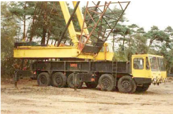
Images - Left - The L1000 was a simple update of the L88-100, the full width tubular steel boom meant the cabin had to be detached for travel. The root section of the boom also had to be detached.
