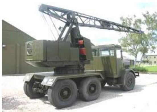
Above - Mk VII EMA petrol-electric crane unit with 5 ton lift, this is fitted to a militarised version of the 6 ton Thorneycroft Amazon 6 x 4 lorry chassis. - now at the Yorkshire Muesum.
