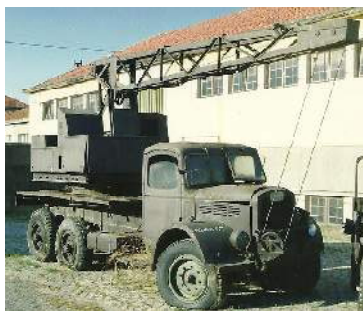
Below - EMA unit fitted to an Austin K6 lorry chassis.
