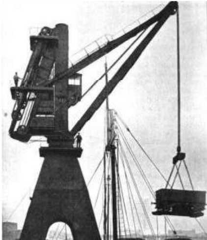
Above - water hydraulic 30Ton 66.ft lift 1915.
